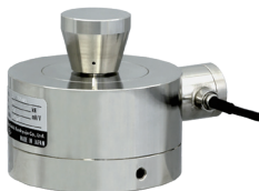
High-precision load cell (Remote sensing compatible)
