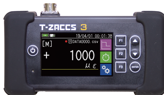
T-ZACCS3 MM-014 strain measurement pocket data logger
