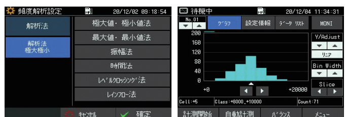
Frequency measurement setting screen and graph display screen using the TMR-381 display unit
